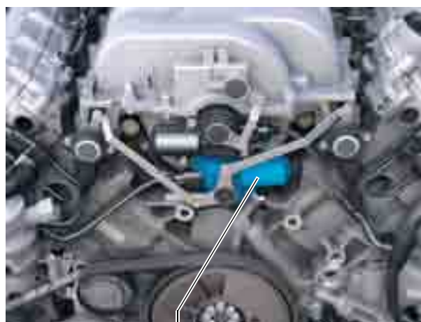
Intake manifold flap motor V157
