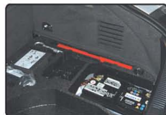
Auxiliary relay carrier below the boot trim
