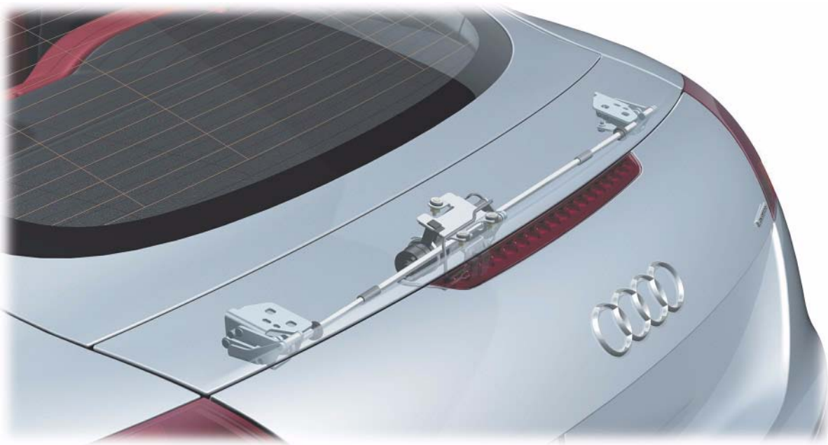
Rear spoiler in lower end position (retracted)
