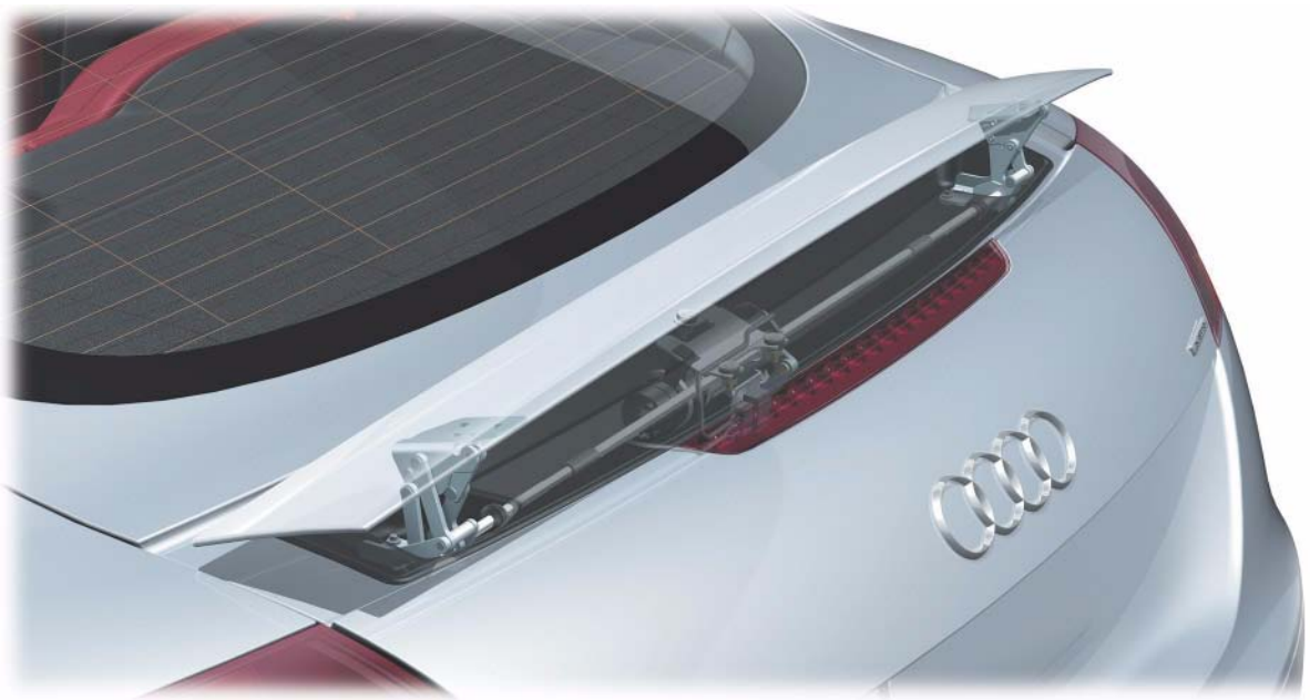
Rear spoiler in upper end position (extended)
