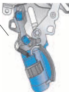
Switch to open convertible left lock F323, F324 and convertible top left lock motor V291
