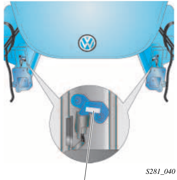
Early crash sensors in longitudinal member
