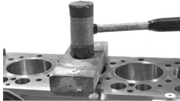
Cylinder Liner Installation
