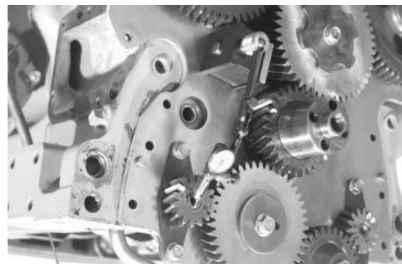
Measuring Balancer Shaft End Play—4-Cylinder
