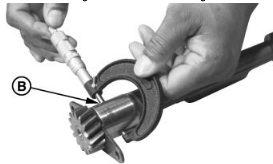
Measuring Balancer Shaft Bushing ID
