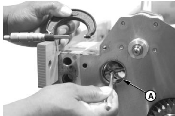
Measuring Balancer Shaft Bushing ID
