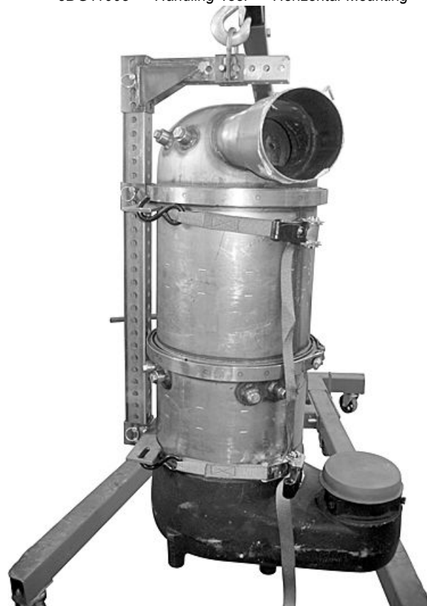
JDG11005 — Handling Tool — Vertical Mounting
