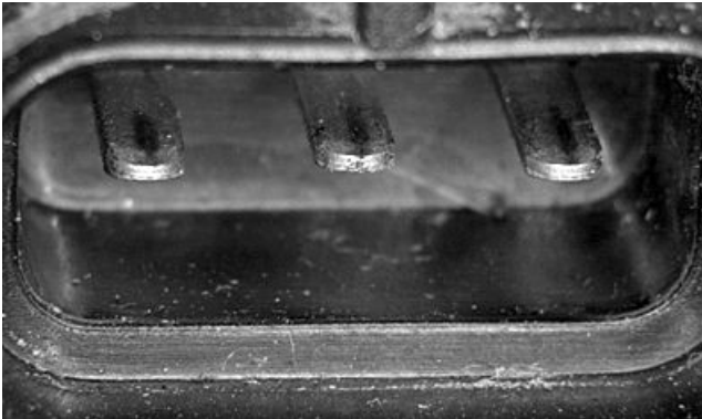
3-pin male- Worn Pins
