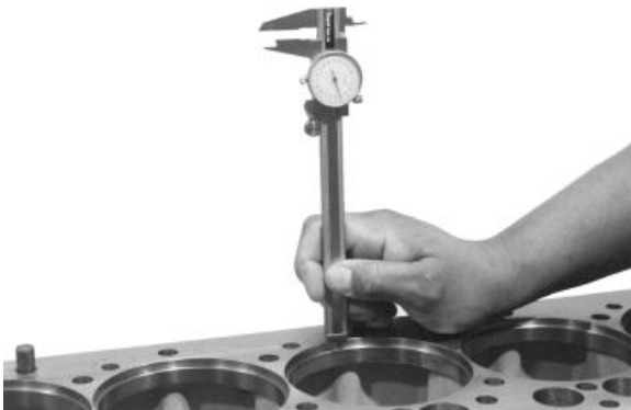
Liner Flange Counter-bore Depth Measurement
