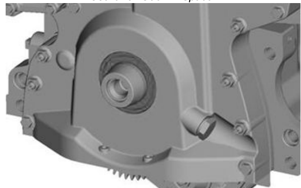
Installed Front Seal
