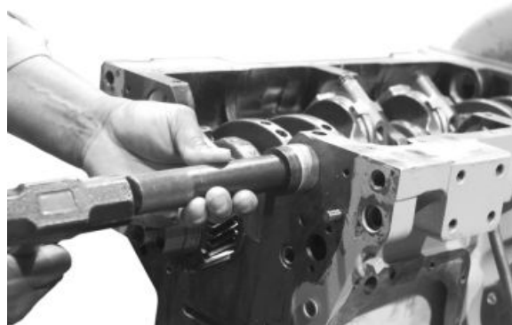
Installing Bushing
