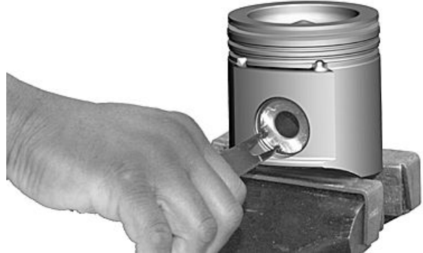
Piston Pin Snap Ring Removal
