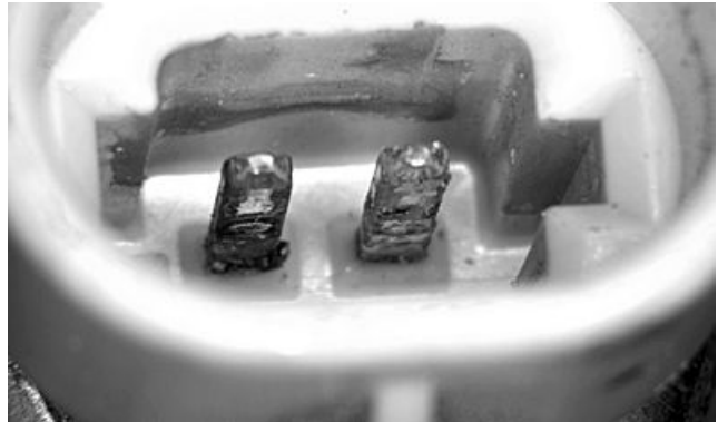
2-pin male- Worn and Corroded Pins
