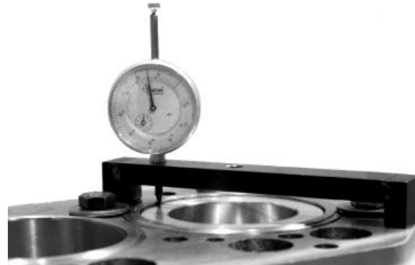
Piston Protrusion Measurement with JDG451
