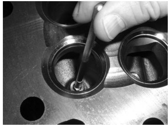
Valve Guide ID Measurement
