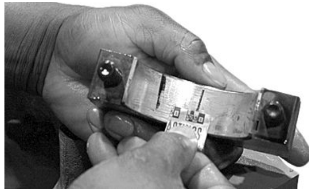
Check Bearing Oil Clearance
