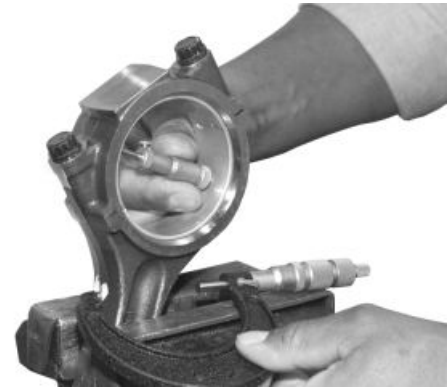
Rod Bearing ID Measurement
