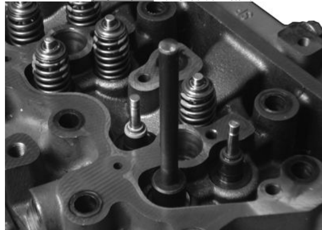
Valve Guide Installation
