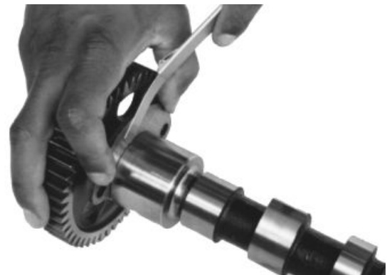
Measure Camshaft Thrust Plate
