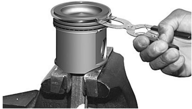
Piston Ring Removal
