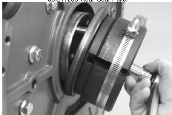
Remove Rear Seal
