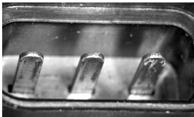
3-pin male- Worn Pins
