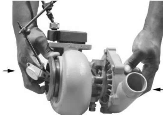
Axial Bearing and End Play Test
