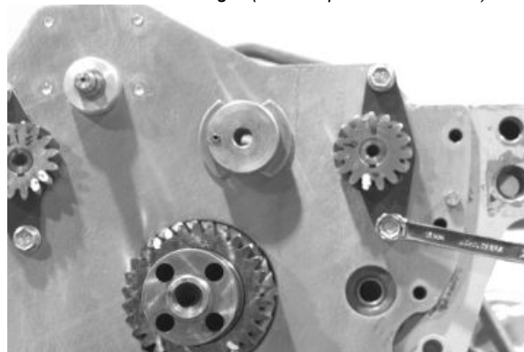
Thrust Plate Cap Screw
