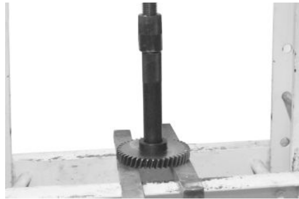
Replace Lower Idler Gear Bushing
