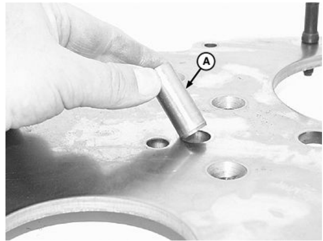
Install Upper Idler Gear Hub Pin
