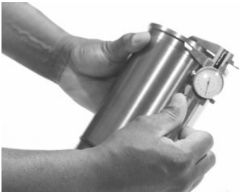
Liner Flange Thickness Measurement
