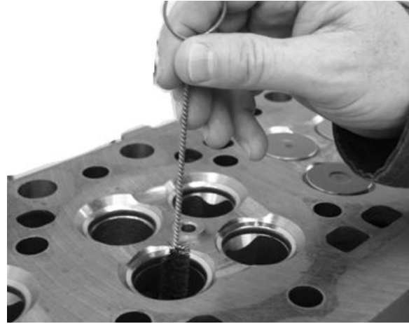
Valve Guide Cleaning
