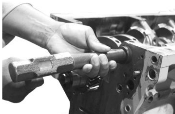
Removing Bushing
