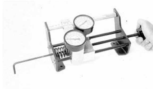
Checking Valve Spring Tension
