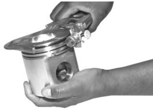
Piston Ring Grooves Cleaning
