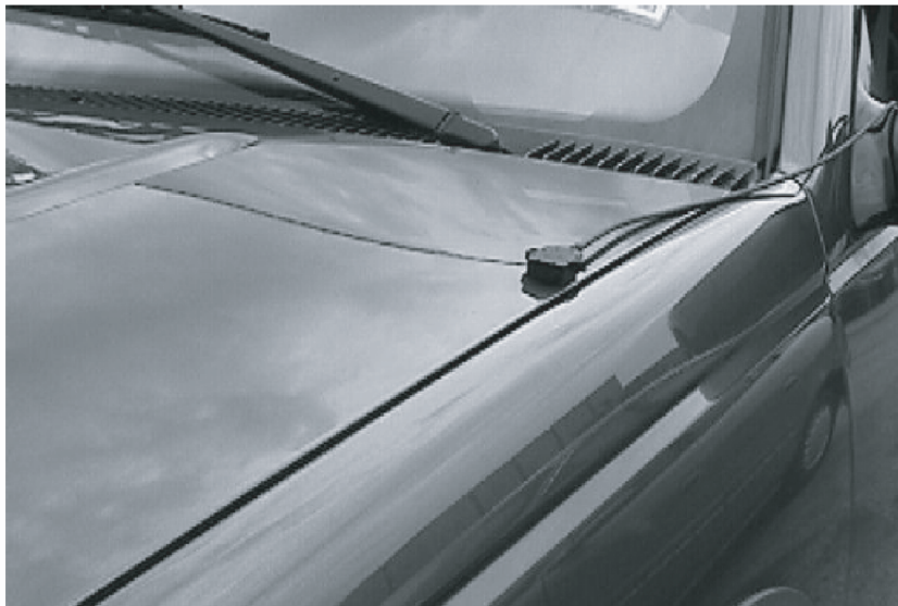
Figure 5-53, Determining Vibration Amplitude
