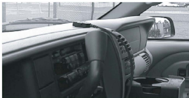
Figure 5-9, Sensor Placement Instrument Panel
