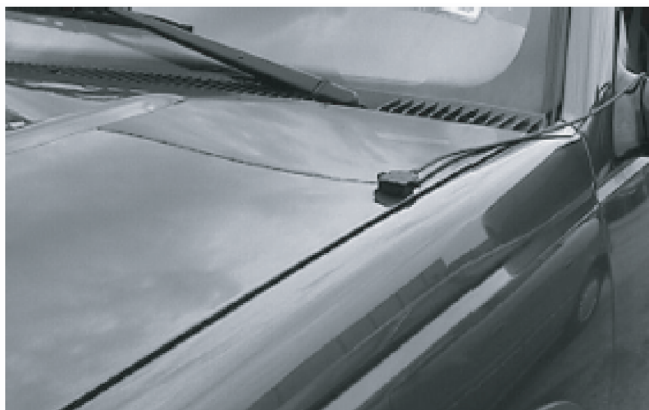
Figure 5-10, Sensor Placement Front Fender
