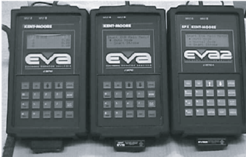
Figure 5-4, Electronic Vibration Analyzer (EVA)
