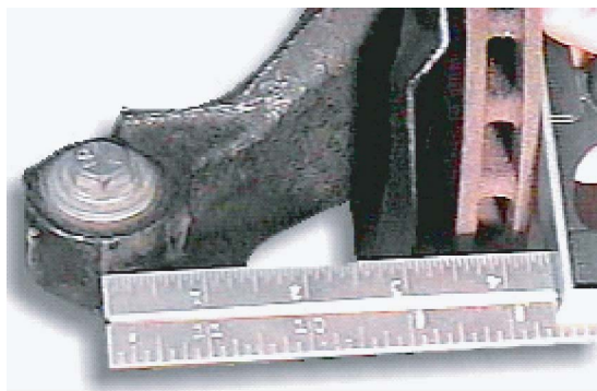
Figure 4-22, Check for Tie Rod or Steering Arm Damage
