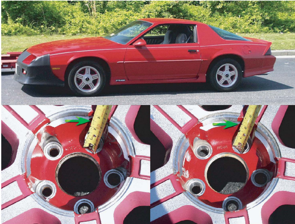
Figure 4b-5, Camaro's Wheels Use A Different Offset From Front-to-Rear
