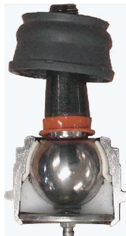
Figure 4b-25, Ball Joint
