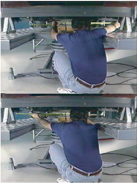
Figure 4b-81, Check for a Bent Control Arm with a Tape Measure
