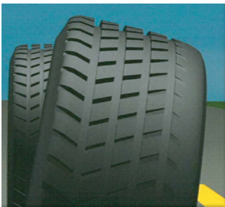
Figure 4b-53, Excessive Camber May Cause Shoulder Wear on the Tire's Tread
