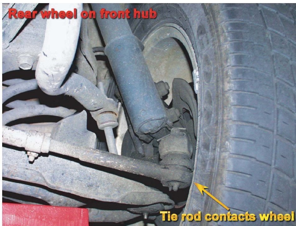
Figure 4b-6, Rear Wheel Hits the Tie Rod When Mounted on the Front Hub
