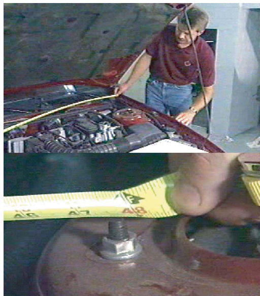
Figure 4b-83, Strut Tower Gauge
