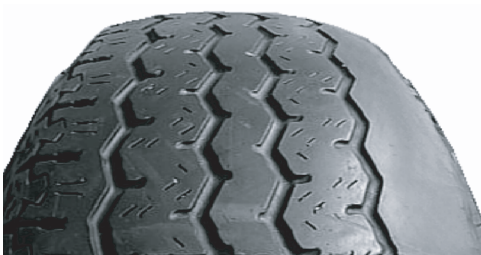
Excessive Camber or Toe
