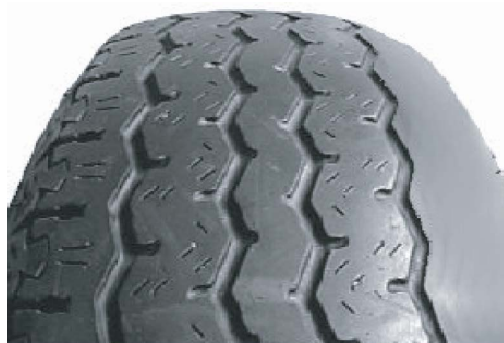
Figure 4-34, Excessive Toe Causes Shoulder Wear on the Tire's Tread
