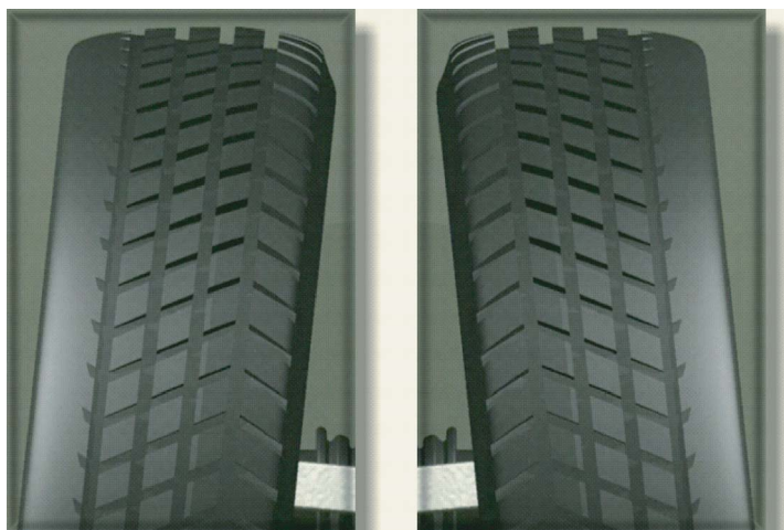
Figure 4b-55, Excessive Toe Causes Shoulder War on the Tire's Tread
