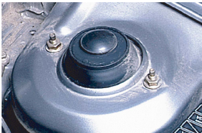
Figure 4b-32, Upper Strut Bearing
