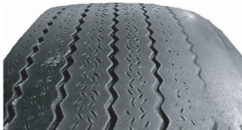
Excessive Front Toe
