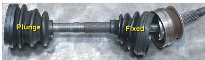
Figure 4b-30, Axle Shaft Assembly
