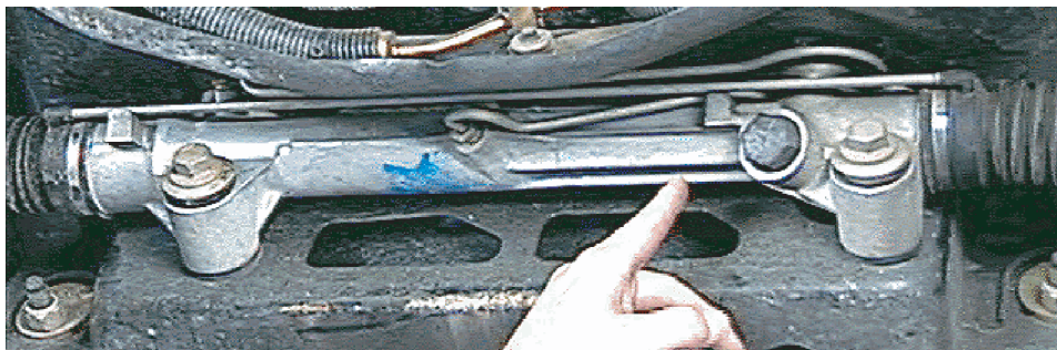
Figure 4b-8, Inspect the Rack Mounting Rubber Insulators
