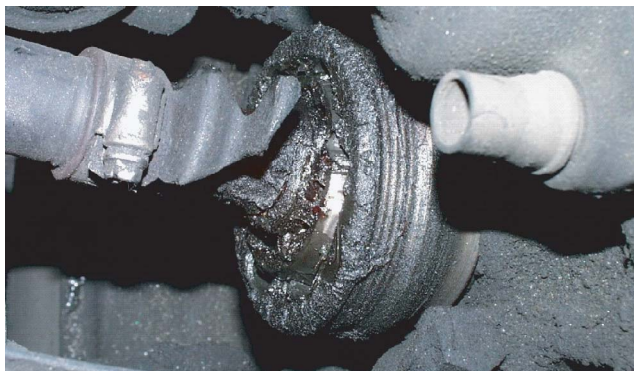
Figure 4b-31, Torn Outer CV Boot
