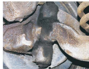
Forged axles with kingpins
