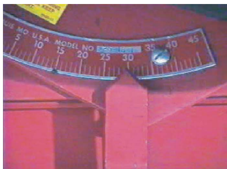
Left wheel turned to the inward lock
