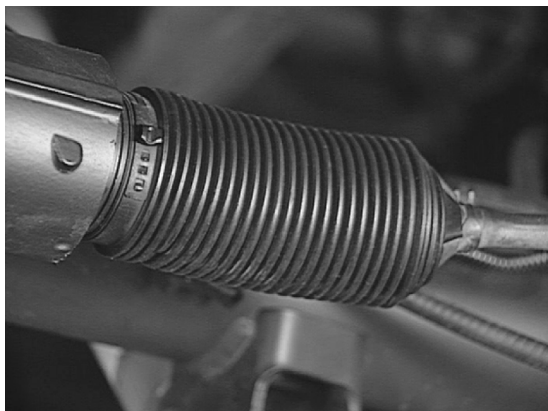
Figure 3-44, Rack and Pinion Boot
