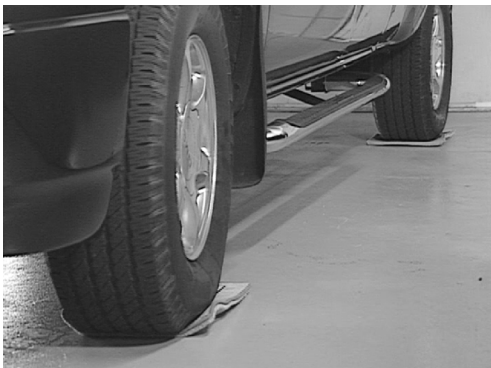
Figure 3-25, 2-Wheel Steer - Wheels Remain Straight
