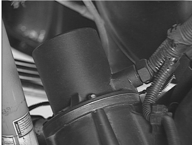
Figure 3-50, Steering Gear Motor
