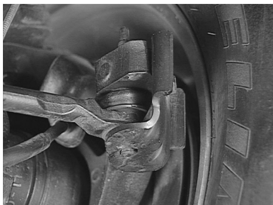
Figure 3-43, Tie Rod Bracket
