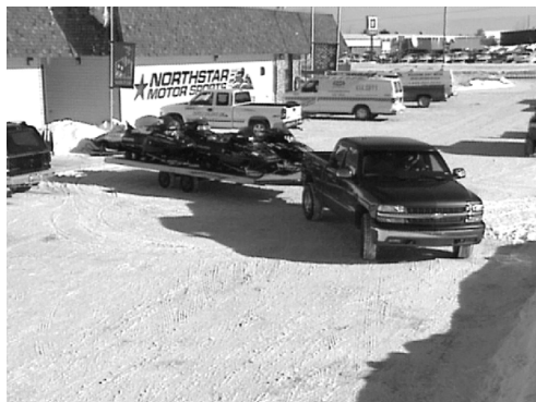
Figure 3-27, 4-Wheel Steer Tow - Positive/Negative Phase
