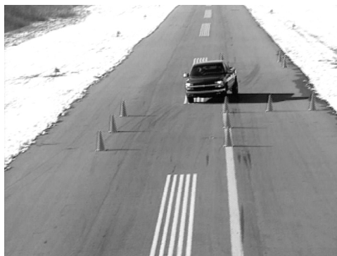
Figure 3-5, Front and Rear Wheels Turned in Same Direction
