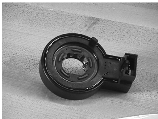
Figure 3-18, Handwheel Position Sensor
