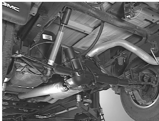
Figure 3-32, Steerable Rear Axle
