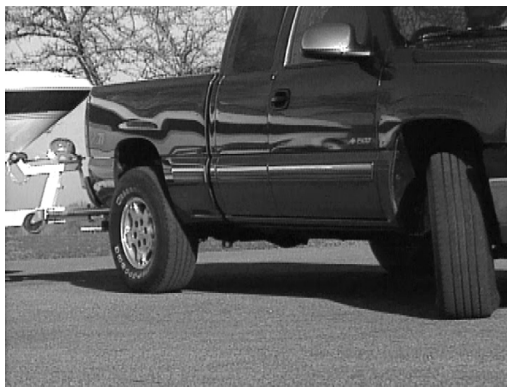
Figure 3-9, Front Wheel and Rear Wheel Turning in Opposite Directions
