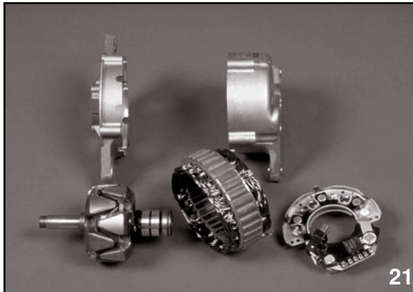
Alternator components
